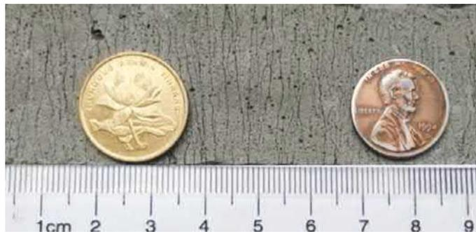
**Figure 2.1:** Multiple cracking in SHCC, from ZHAN et al. [120].
