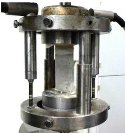
**Figure 12.1:** The testing setup for the quasi-static tensile test with SHCC, from CUROSU [24].
