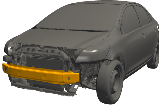
Figure 1.1: Highlighted in orange, a normally hidden car front bumper, shown by means of a Toyota Yaris. The overall objective of this thesis is the optimization of the performance of such a front bumper in a crash scenario, considering polymorphic uncertainties.
