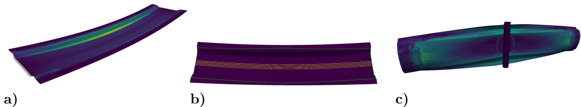
Figure 7.3: The three investigated steps, a) deep-drawing of the sheet metal, b) trimming and spring back and c) simple frontal crash. The images are taken from Miska and Balzani [98].
